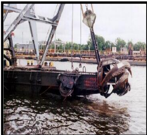
Figure 5-1. Cutterhead pipeline dredge schematic.
